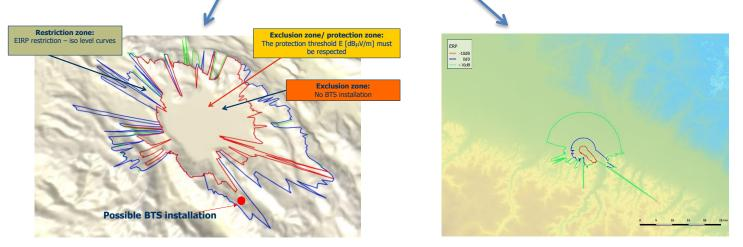
areas delimited by the iso-line curves where the incumbent protection criteria based on I/N is respected for a specific BTS EIRP value
