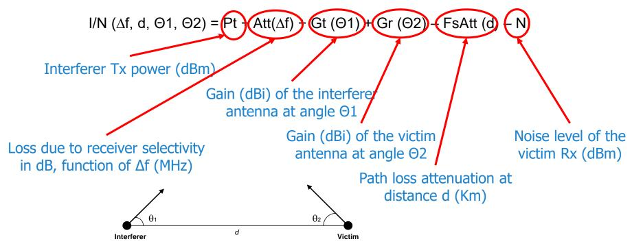
The value of I/N is compared with the threshold at the victim receiver
